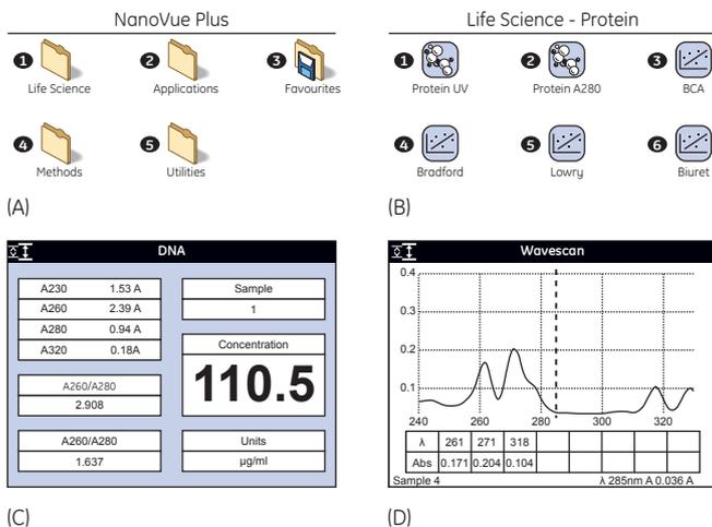
**Fig 3.** NanoVue Plus spectrophotometer screenshots showing; (A) Simple interface for easy selection of applications; (B) Protein methods interface; (C) DNA quantitation results and (D) An example of a wavelength scan.
